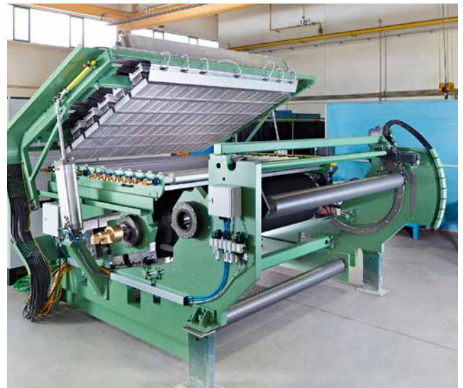
KRELUS infrared preheating for embossing machines Source: Kampf LSF GmbH, Laussig, Germany
