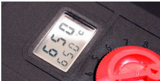
SYSTEM: Digital display of nominal and current values
