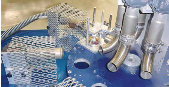
High-end air heaters on an indexing table for producing light bulbs.
