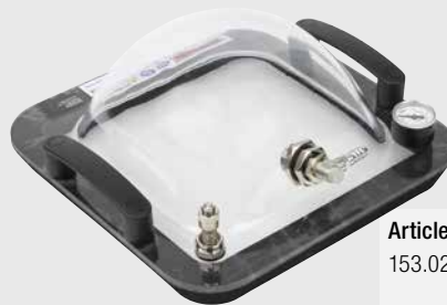
For testing T-joints
