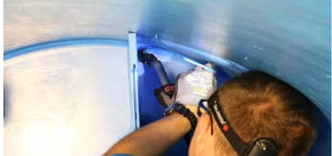
WELDING PEN R, combined with angle adapters, make welding possible even in very tight spaces.
