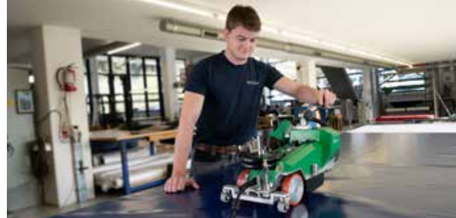
UNIPLAN 300 / UNIPLAN 500: ideal for overlap, hem, and pipe welding either on a table or on the ground.
