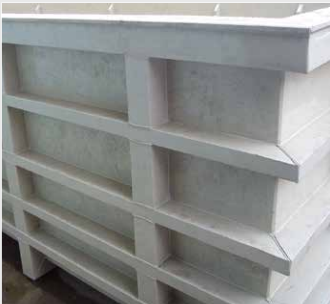
Electroplating tank, Turkey. Material: PP
