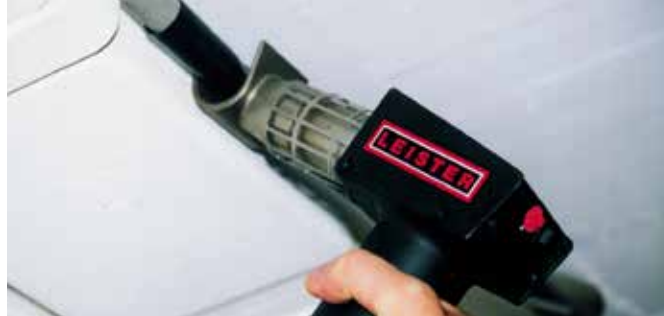
Shrinking cable connections with the GHIBLI.
