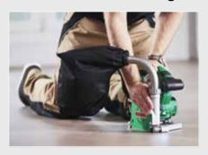
**Step 1:**Milling the groove with the GROOVER.
