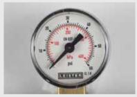
Manometer ASTM (psi/kPa)
