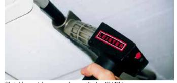
Shrinking cable connections with the GHIBLI.
