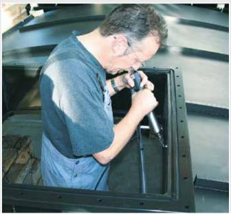
DIODE S for use with draw welding on a tank detail.
