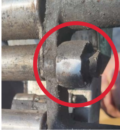
Heavy dirt Heavy dirt buildup causes bearing to be blocked and inhibited
