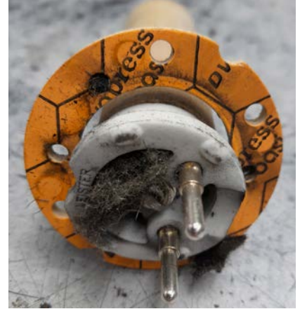
Filter not installed
