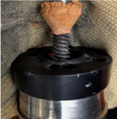
Incorrect handling: Two welding wires were inserted together, causing the plastic to be pushed back.
