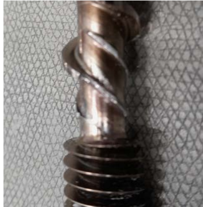
Incorrect handling: Small stones were drawn in with the welding wire and damaged the screw.
