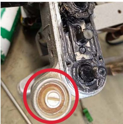
Corrosion of moving parts
