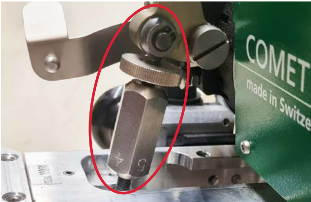
Bent pressure adjustment screw due to excessive joining pressure in GEO devices (image does not show damage)
