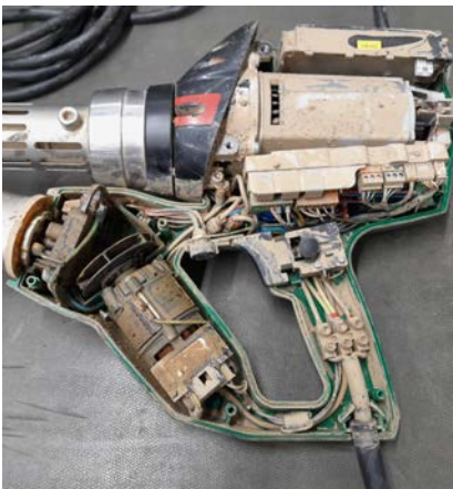
Lack of maintenance, device very dirty
