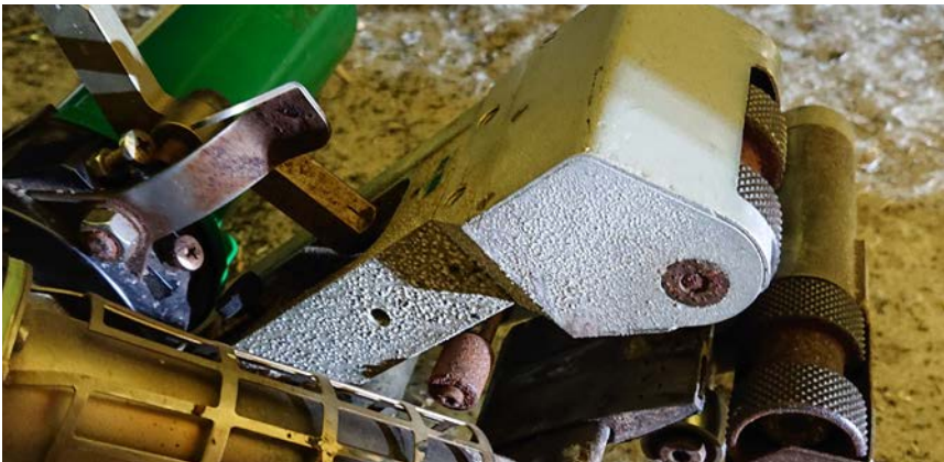
Corrosion caused by welding of PVC
