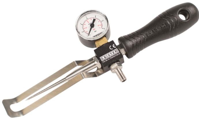
The Leak tester is a reliable compressed air testing device for checking the tightness of overlap seams with test channel. Developed for quality assurance of weld seams in civil engineering, tunnels and landfill sites.
