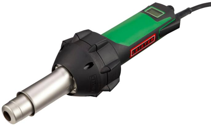
The TRIAC AT heat gun is designed to weld and mold plastic. The temperature and air quantity can be set separately by means of its e-Drive control unit.
