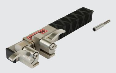
The EXAMO 100 tensile tester tests the weld seam quality of geomembranes. Advantages: tool-free clamping of the specimens, constant tensile speed as well as effortless pulling of the specimens with the cordless screwdriver.
