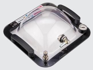
VACUUM BELL is a practical, plastic vacuum bell. It is especially used in landfill engineering and tunnel construction to ensure overlap welding seams are leak-proof.
