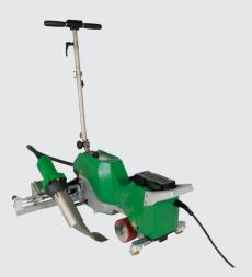
The VARIANT 700's modular design converts from overlap to tape welding and welds up to 20 m/min, ideal for tarpaulins, tents, and banners. Plug-and-play wheels, lift-and-weld technology, and Eco Mode enhance efficiency.
