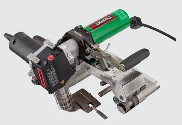
The welding machine TWINNY S with combination wedge is designed in particular for overhead welding in tunnel construction. In the process, it welds thin geomembranes made of PVC, HDPE and LDPE very reliably and safe.
