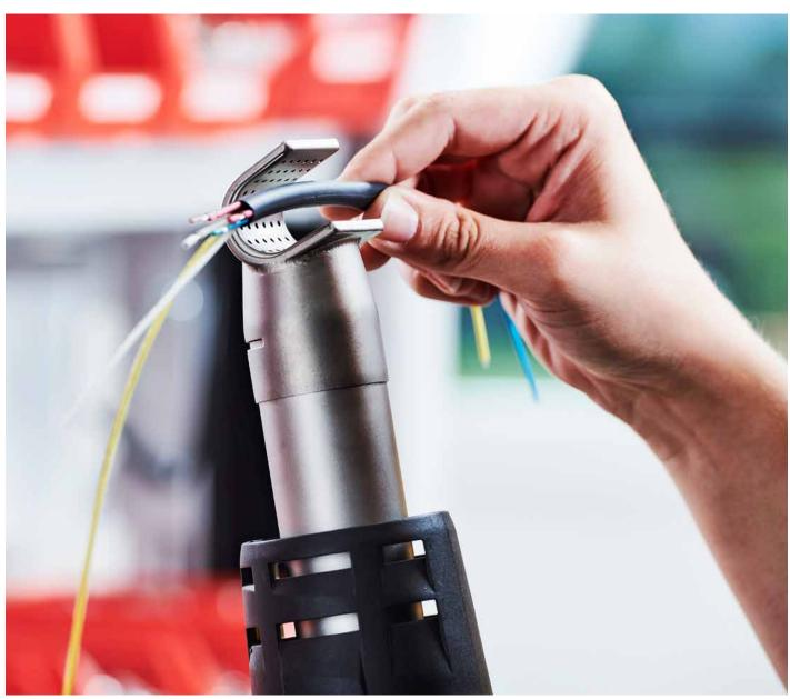
Cable shrinking procedure with the SOLANO AT from Leister
