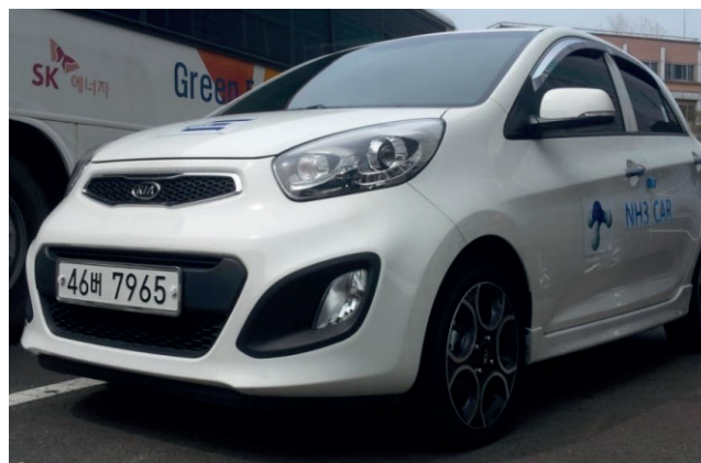
A small car powered by ammonia and gasoline – the result of KIER's AmVeh project
